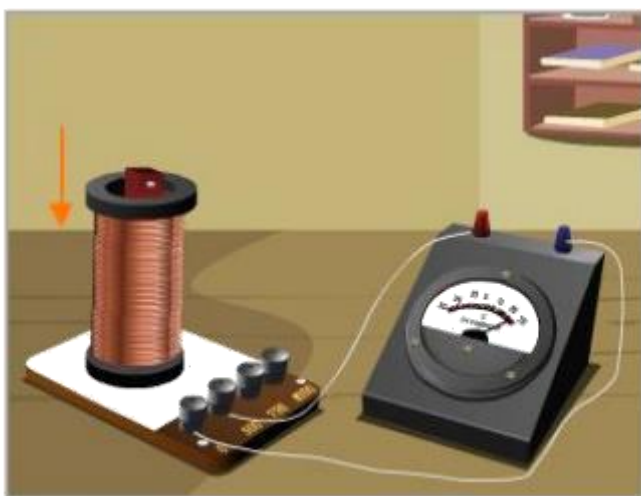
The North pole of the magnet is moved into the coil of wire
