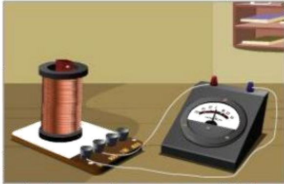
The Magnet is Held Stationary Inside the Coil of Wire
